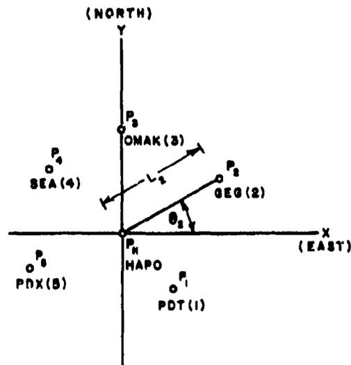
With use of the sea-level pressure reported for each of the stations shown in Fig. III-1, the representative pressure gradient across Hanford was determined by resolving the east-west and north-south components of the pressure gradients between Hanford and each of the other five stations, and then summing these components.
