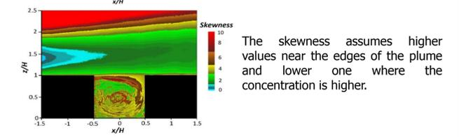
The skewness assumes higher values near the edges of the plume and lower one where the concentration is higher.
