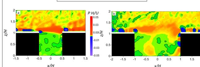
The production term  $P$  is defined  $P = -\overline{u'_i u'_j \frac{\partial \bar{u}_i}{\partial x_j}}$  ( $i=1,2,3$   $j=1,2,3$  indicate the axis of the coordinate system). It is positive above the canyon top particularly for  $AR=1$  (a), where the region of maxima corresponds with the mixing, characterized by strong vertical shear. For  $AR=2$  (b) the region of maxima is still present, even though it is less evident.
