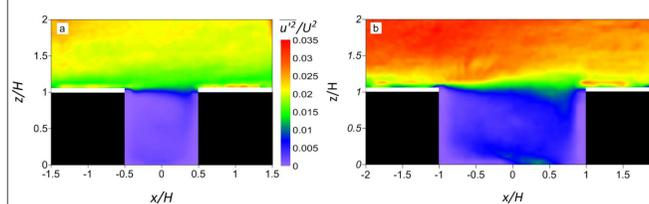
According to other works reported in the literature, the variance of the non-dimensional horizontal velocity components,  $u'^2/U^2$  (here primes are fluctuations around the mean) assumes lower values inside the canyon (nearly one order of magnitude) irrespective of AR.
