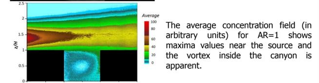
The average concentration field (in arbitrary units) for  $AR=1$  shows maxima values near the source and the vortex inside the canyon is apparent.
