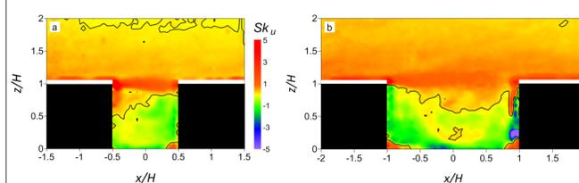
$Sk_u = \overline{u'^3}/(\overline{u'^2})^{3/2}$  for  $AR=1$  (a) and 2 (b) is negative almost everywhere inside the canyon for both ARs, except near the canyon top, where, for  $AR=1$ , a region of large, positive  $Sk_u$  is present. For  $AR=2$ , large (positive) values are located also near the buildings top. The skewness factor of the vertical velocity component has been calculated too, but is not presented here.
