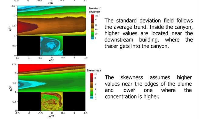
The standard deviation field follows the average trend. Inside the canyon, higher values are located near the downstream building, where the tracer gets into the canyon.
