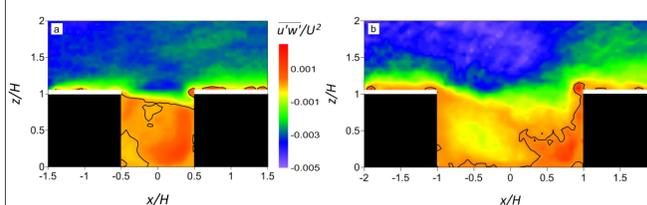
The non-dimensional, vertical momentum flux  $\overline{u'w'}/U^2$  is negative above the canyon for both the configurations, while, inside, it strongly depends on AR. In fact, for  $AR=1$  (a) it is positive almost everywhere while, for  $AR=2$  (b), it is positive only near the bottom right corner of the canyon.
