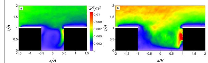
The non-dimensional vertical velocity variance,  $w'^2/U^2$ , shows large values within a tongue-like feature, coming from the outer flow, near the windward wall when  $AR=1$  (a). That feature is much more large for  $AR=2$  (b), where in the right-half of the canyon  $w'^2/U^2$  is of the same order of that present in the outer flow.
