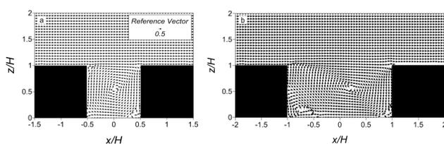
Velocity components are expressed as  $\bar{u}/U$  and  $\bar{w}/U$ . For  $AR=1$  (a) the vortex is slightly shifted downstream and towards the top of the canyon and, at the bottom-right corner of the canyon, a little counter-rotating vortex is present. For  $AR=2$  (b), instead, the main vortex is significantly shifted downstream and a well-defined counter-rotating vortex form near the leeward building.
