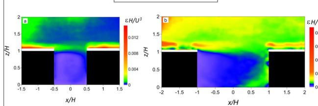
The rate of dissipation of TKE,  $\epsilon$ , is estimated as  $\epsilon = \frac{15}{4} \nu \left[ \left( \frac{\partial \bar{u}}{\partial z} \right)^2 + \left( \frac{\partial \bar{w}}{\partial z} \right)^2 \right]$ . Lower values occur for both ARs within the canyon, particularly near the leeward building. Above the canyon,  $\epsilon$  reaches higher values, with peaks above the rooftops.
