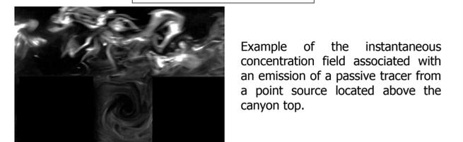
Example of the instantaneous concentration field associated with an emission of a passive tracer from a point source located above the canyon top.
