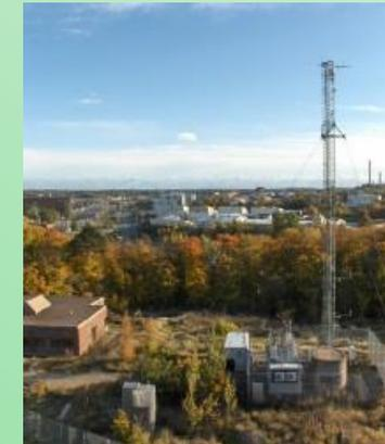
SMEAR III - 31 m tower 4 km from down town Helsinki instrumented at several heights yielding profiles of temperature wind radiation components
