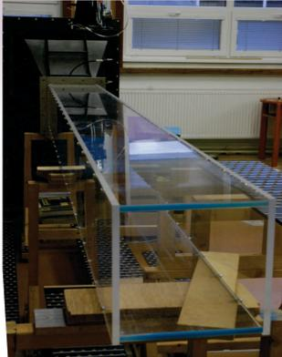
Figure 2: Scheme of the wind channel: Cross-section 0.25 m x 0.25 m. Reference wind speed 5 m/s.
