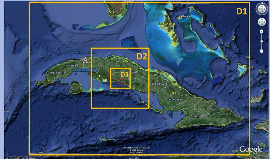
Figure 3. Nested WRF simulation domains (resolution: D1: 27x27 km<sup>2</sup>; D2: 9x9 km<sup>2</sup>; D3: 3x3 km<sup>2</sup>), to provide meteorological inputs to CALMET model domain (□: 1x1 km<sup>2</sup> resolution).
