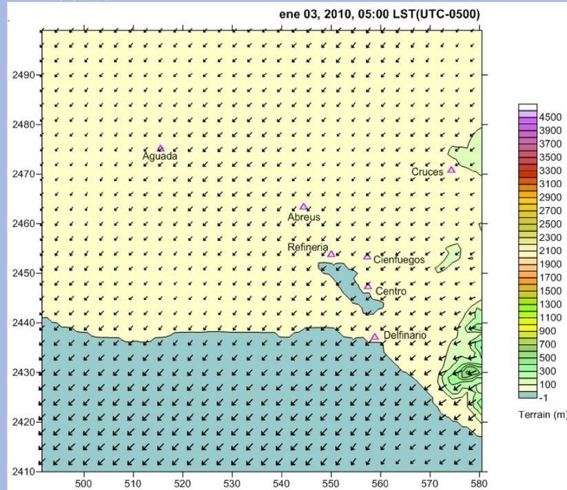
Figure 2. Surface wind field from Met\_1 CALMET simulation at 3/Jan/2010 05LST over Jagua Bay, and location of 7 surface meteorological sites applied.
