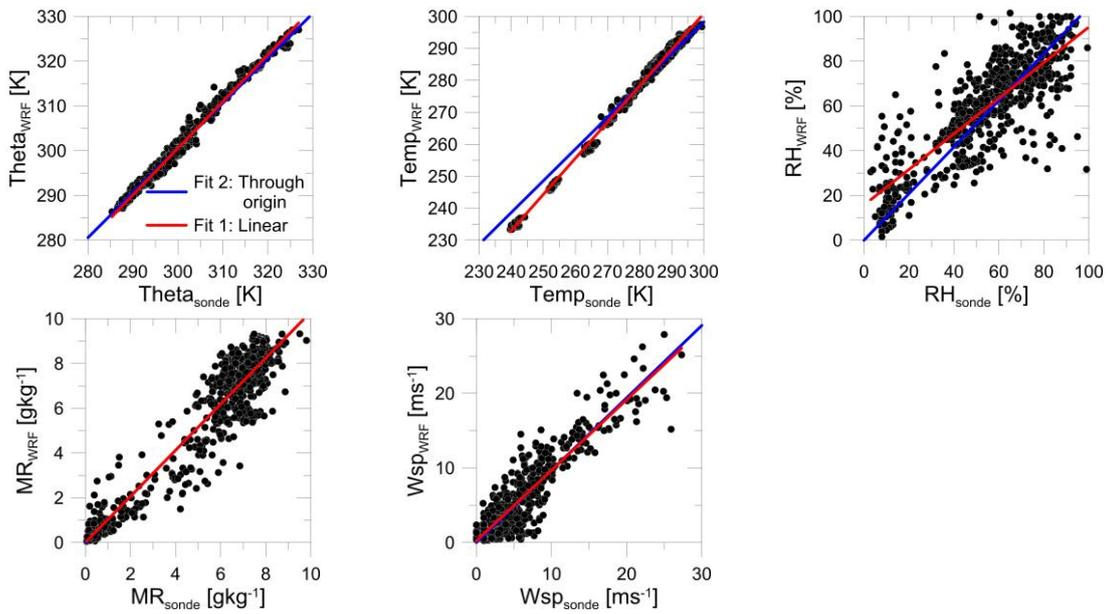
**Figure 2.** Scatter plots of Theta, Temp, RH, MR, Wsp for all radiosoundings and all levels up to 8000 m
