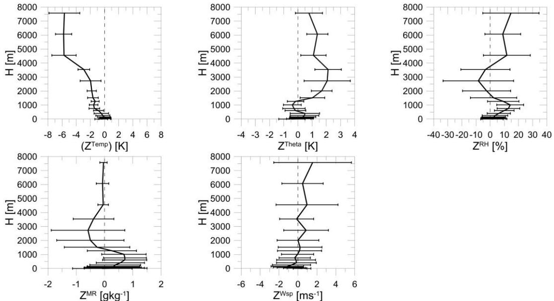
**Figure 3.** Averaged value of Z ( $Z = \text{Value}^{\text{WRF}} - \text{Value}^{\text{Sonde}}$ ) from all 35 soundings and its SD for each model level up to 8000 m
