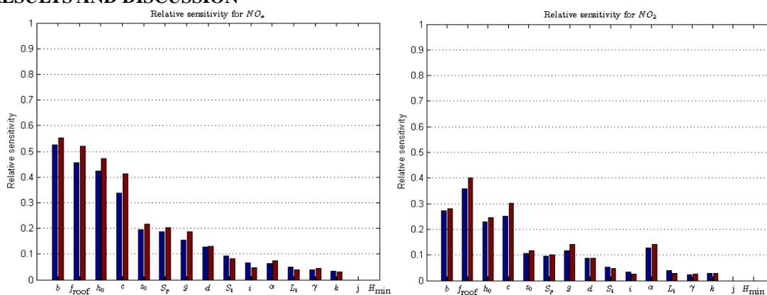
**Figure 2.** Root mean square local sensitivity for the DUPLEX estimation set (blue) and the Seasonal estimation set (red) for respectively  $\text{NO}_x$  (left) and  $\text{NO}_2$  (right).
