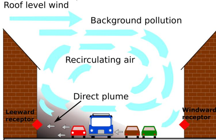
**Figure 1.** Schematic illustration of the direct and recirculating component of the concentration in OSPM. Figure modified from (Silver, Ketzel, and Brandt 2013).
