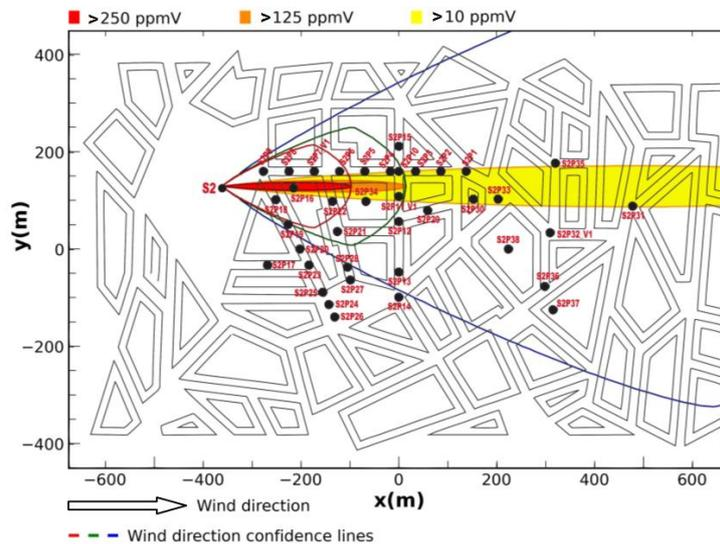
**Figure 1.** Horizontal distribution of average near ground concentrations for a continuous release from source S2 simulated with a models of type I (model 101).
