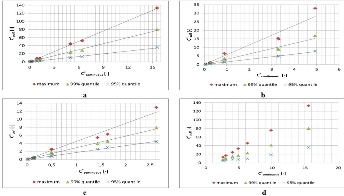
**Figure 7.** Relationship between mean dimensionless concentration for continuous source and mean maximum, mean 99% and mean 95% quantile of dimensionless concentrations for puff source within separate traverse streets (a corresponds to the first, b to the second, c to the third traverse street) and within the plume axis (d).
