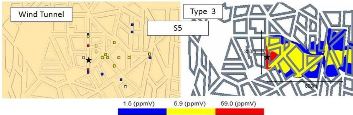
**Figure 2.** Sketch of the Michelstadt continuous release configurations (left) and examples of concentration contours simulated by one model from type 3 (right) as in Table 1, for source S5.
