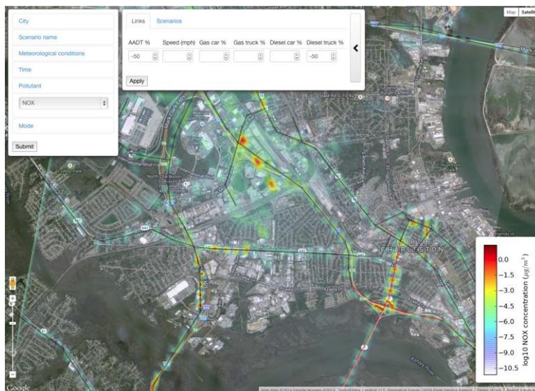
**Figure 2.** Screen shot of C-PORT showing ability to choose road-links on demand (highlighted in red), and changing fleet activity.
