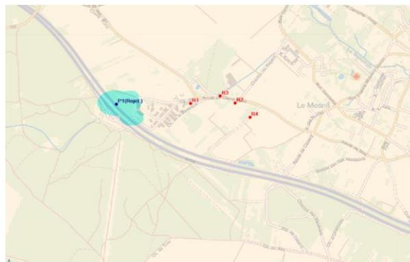
**Figure 7.** Results given by CERES® retro-plume module for an academic case. R1, R2, R3 and R4 are the sensors.
