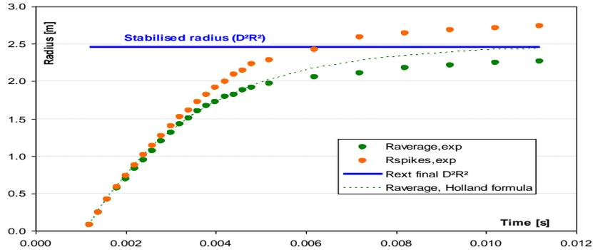
Figure 3. Experimental average and maximum radii for water compared with  $D^2R^2$  prediction and Holland formula.
