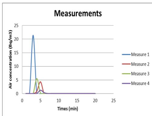
**Figure 6.**  $^{241}\text{Am}$  activity concentration measurements (in  $\text{Bq}\cdot\text{m}^{-3}$ ) on the 4 sensors.
