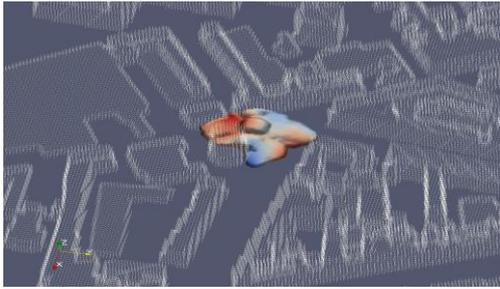
**Figure 5.** Outer boundary of the dispersion cloud for a urban scenario (gas pressure colour-scale).
