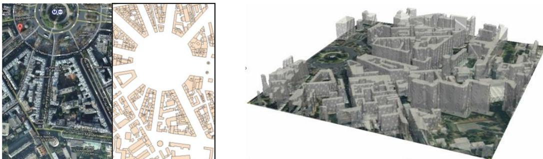
Figure 4. From left to right: Google Maps® view, BD TOPO shapefile, and HI2LO geometry after processing.
