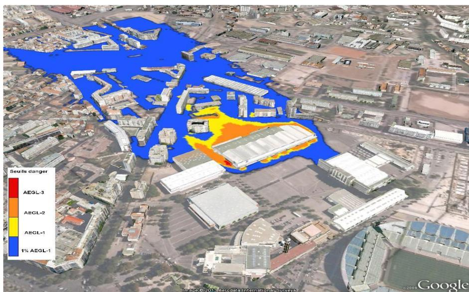
Figure 7. Danger zones corresponding to the AEGL thresholds.
