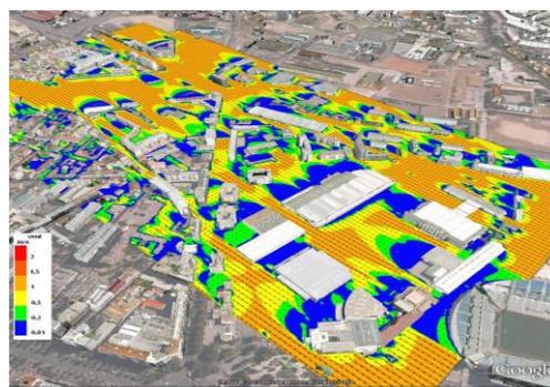
**Figure 5.** Wind field view at 2 m above the ground.
