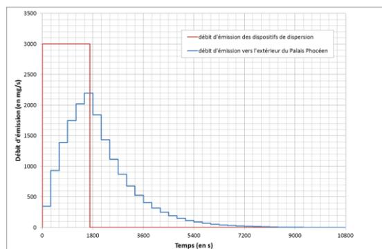
**Figure 4.** Yperite rate release (in  $\text{mg.s}^{-1}$ ) within the dispersal device and to the atmospheric environment.
