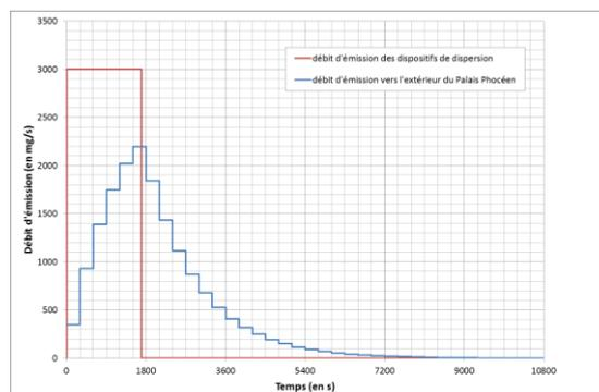
**Figure 4.** Yperite rate release (in  $\text{mg.s}^{-1}$ ) within the dispersal device and to the atmospheric environment.
