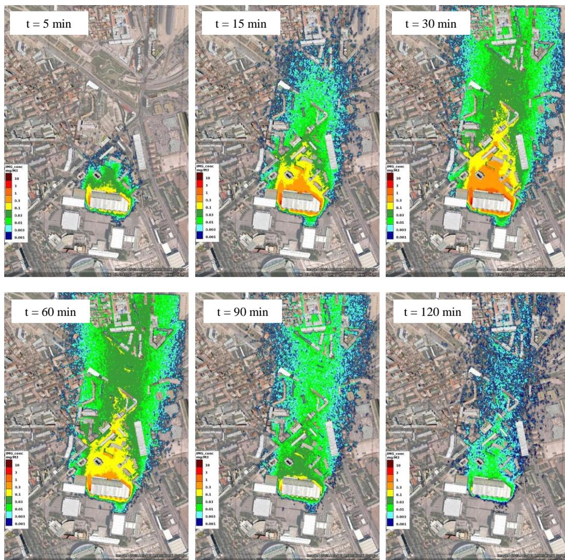
**Figure 6.** Section at 2 m above the ground of the yperite concentration (in  $\text{mg}\cdot\text{m}^{-3}$ ) in the urban district at six instants after the start of the chemical release.
