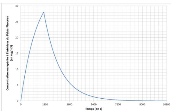
**Figure 3.** Yperite concentration (in  $\text{mg.m}^{-3}$ ) evolution inside the exhibition hall.
