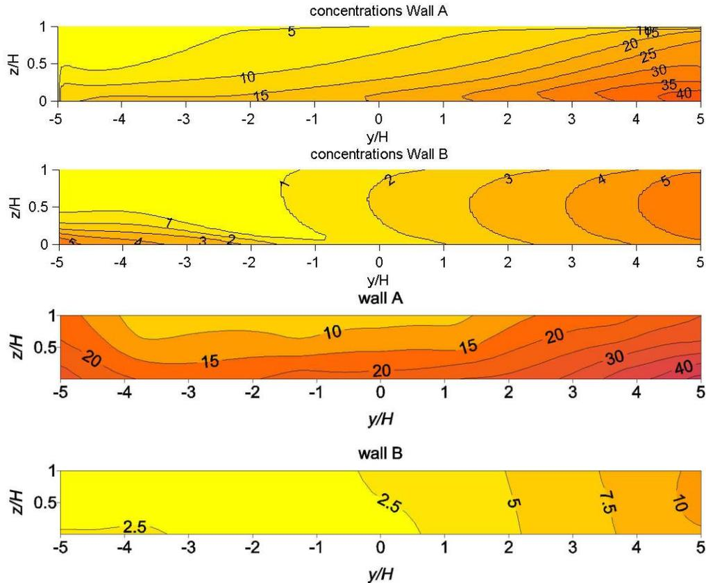
**Figure 1.** Normalized concentration profiles inside the street canyon near the walls of both buildings for  $W/H = 1.0$ ,  $45^\circ$ , no trees. Top two profiles are from the CFD simulations, bottom two reproduced from CODASC, 2008.
