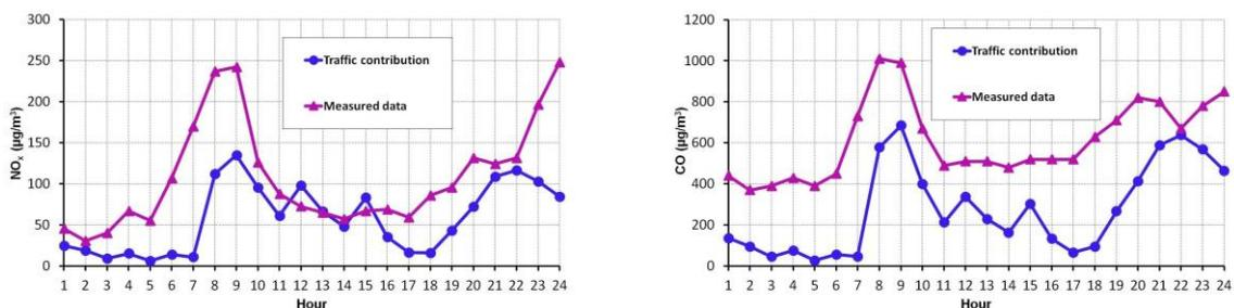
**Figure 3.** Daily patterns of hourly average simulated and measured concentrations for NO<sub>x</sub> (left) and CO (right) at the measuring site. Data refer to 28<sup>th</sup> March 2007.
