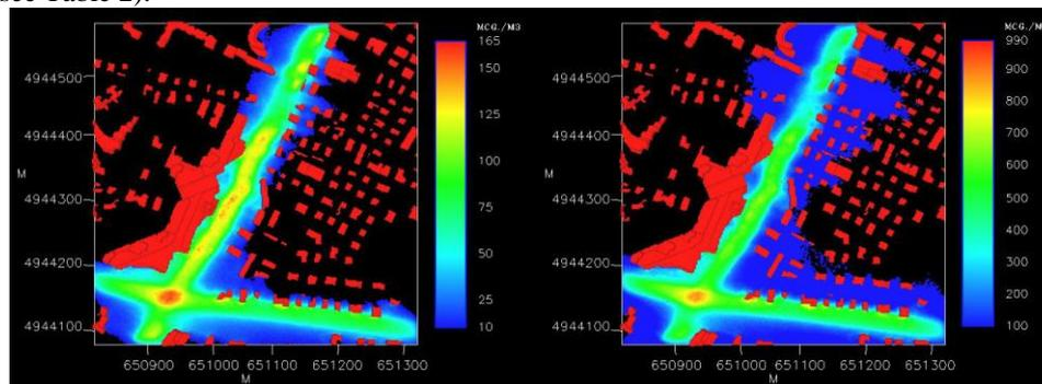
**Figure 2.** Average daily concentration map in the first atmospheric layer for NO<sub>x</sub> (left) and CO (right) traffic emissions.
