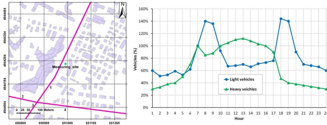
**Figure 1.** Left: simulation domain map (UTM WGS84): measuring station (E = 654 069 m, N = 4 944 284 m) and road sources (1, 2, 3, 4) for traffic emissions. Right: hourly modulation pattern for traffic intensity (light and heavy vehicles) in typical workday (in percent of the number of vehicles of the same category passing from 7:00 to 8:00).
