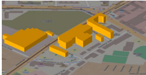
Figure 6. Definition of buildings (cubic elements) on the base of OpenStreetMaps in LASAIR in a city center
