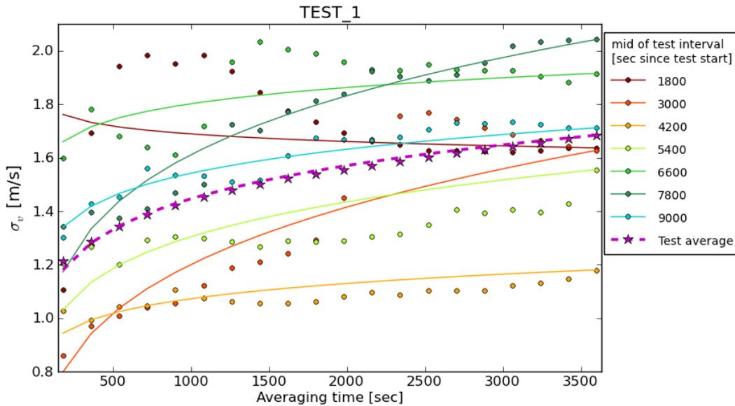
**Figure 3** Experimentally derived  $\sigma_v$  (bullets) and fit (solid line) over averaging time. Individual time slices show no evidence for a power law dependence. However, looking at the test's average (stars), the power law fits the data well (dashed line).
