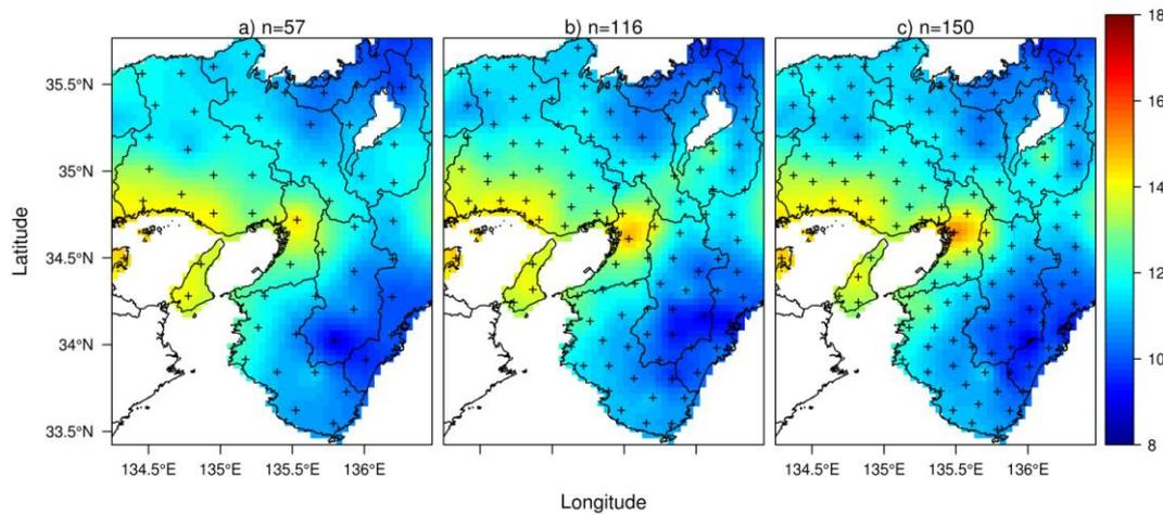
**Figure 2.** The optimized network by the HGS for the network size a)  $n=57$ , b)  $n=116$  and c)  $n=150$ . The concentration fields are generated by ordinary kriging with the simulated values at the selected sites. The crosses represent the selected sites. Unit is  $\mu\text{g m}^{-3}$ .
