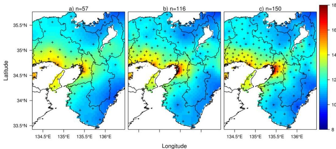
**Figure 3.** The optimized network by the HGS with the concentration based weighing factor for the network size a)  $n=57$ , b)  $n=116$  and c)  $n=150$ . The concentration fields are generated by ordinary kriging with the simulated values at the selected sites. The crosses represent the selected sites. Unit is  $\mu\text{g m}^{-3}$ .
