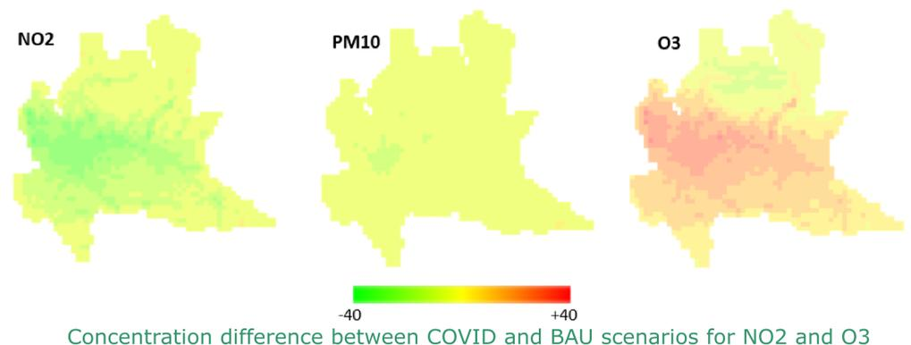
Concentration difference between COVID and BAU scenarios for NO<sub>2</sub> and O<sub>3</sub> in ppb and PM<sub>10</sub> in µg m<sup>-3</sup>
