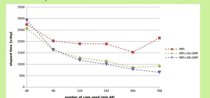
Figure 1- Calculation speed (elapsed time) in seconds per day for the simulation with a horizontal spatial resolution of 4x4 km.
