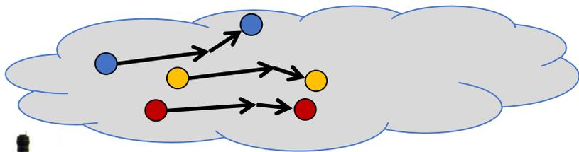
Discretization of the plume into virtual particles, each carrying a fraction of the emitted mass
