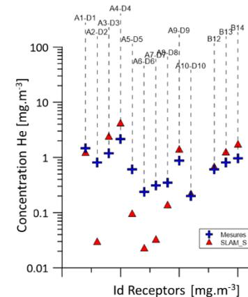
Scatter plot of measures and result of SLAM\_S for one scenario on campaign 1 (a) and comparison point to point for each captor EA of IRSN used during experiment (b)
