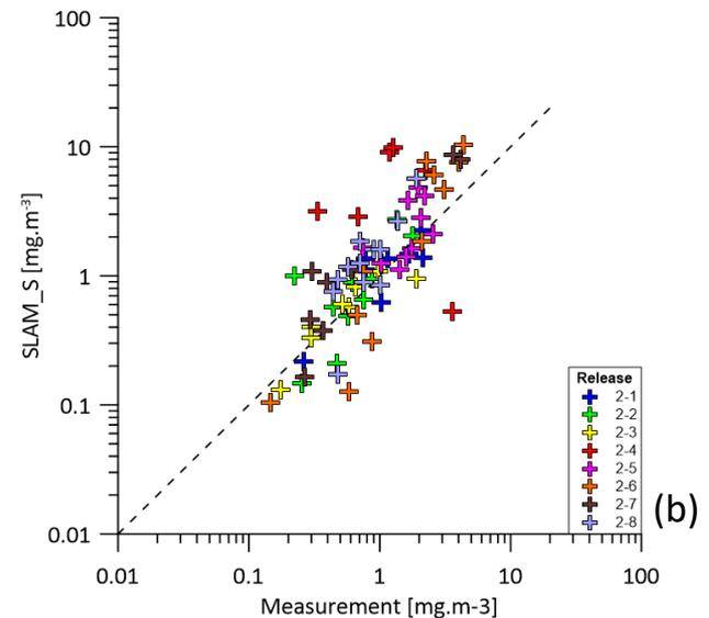
*Comparison of concentrations measured and modelled with SLAM\_S, using meteorological data provided by the anemometer H, for campaign 1 (a) and campaign 2 (b)*
