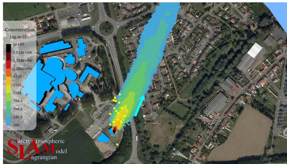
*Helium concentration field on the ground calculated by SLAM\_S ( $\mu\text{g.m}^{-3}$ )*
