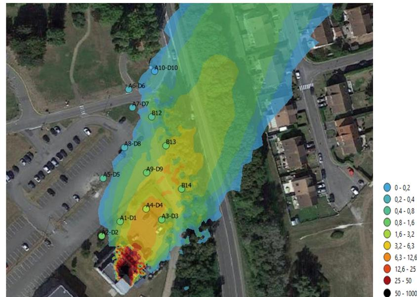
*Focus on Helium concentration field on the ground calculated by SLAM\_S ( $\mu\text{g}\cdot\text{m}^{-3}$ ) and value measures on captor during experiment (dot)*
