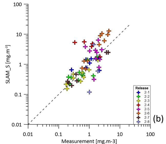
*Comparison of concentrations measured and modelled with SLAM\_S, using meteorological data provided by **LIDAR**, for campaign 1 (a) and campaign 2 (b)*
