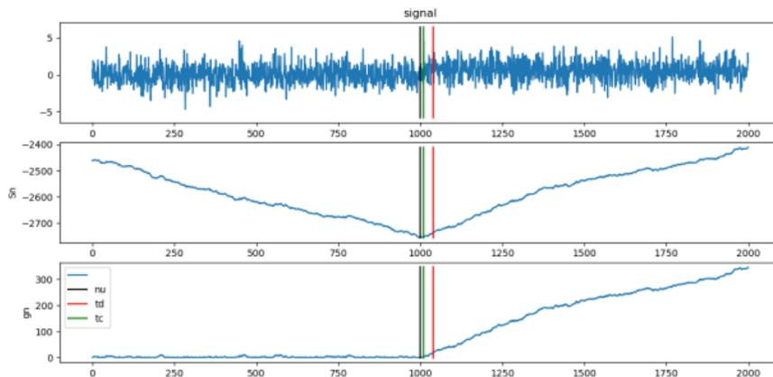
**Figure:** Example of CUSUM at low SNR (-15dB): 'nu' shows the real value of  $\nu$ , 'td' is time of detection and 'tc' the estimate of the change-point time.
