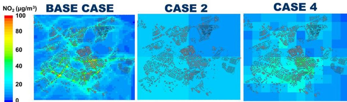
**Figure 2.** Maps of annual average NO<sub>2</sub> at different spatial resolutions. Base case at 100 m x 100 m, Case 2 at 3000 m x 2500 m and Case 4 at 500 m x 500 m.
