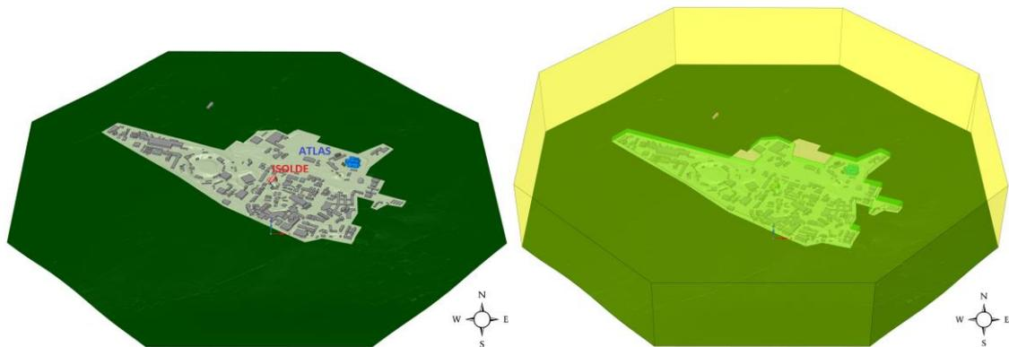
**Figure 1.** Polyhedral shaped domain including topography model (olive and dark green ground), CAD buildings (grey, red and blue buildings), body of interest (transparent light green volumes) and walls (transparent yellow walls).
