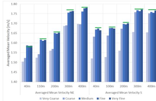
**Figure 5.** Normalized averaged mean velocity plots showing the differences of the values for each plane and wind direction.
