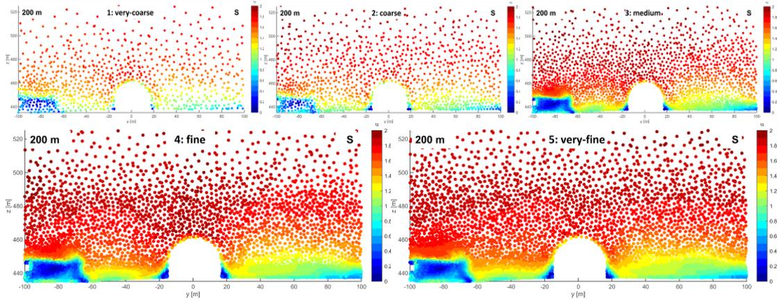
**Figure 3.** Mean velocity magnitude coloured on perpendicular planes. Example for all mesh sizes in south wind direction at 200 m distance from the release point.
