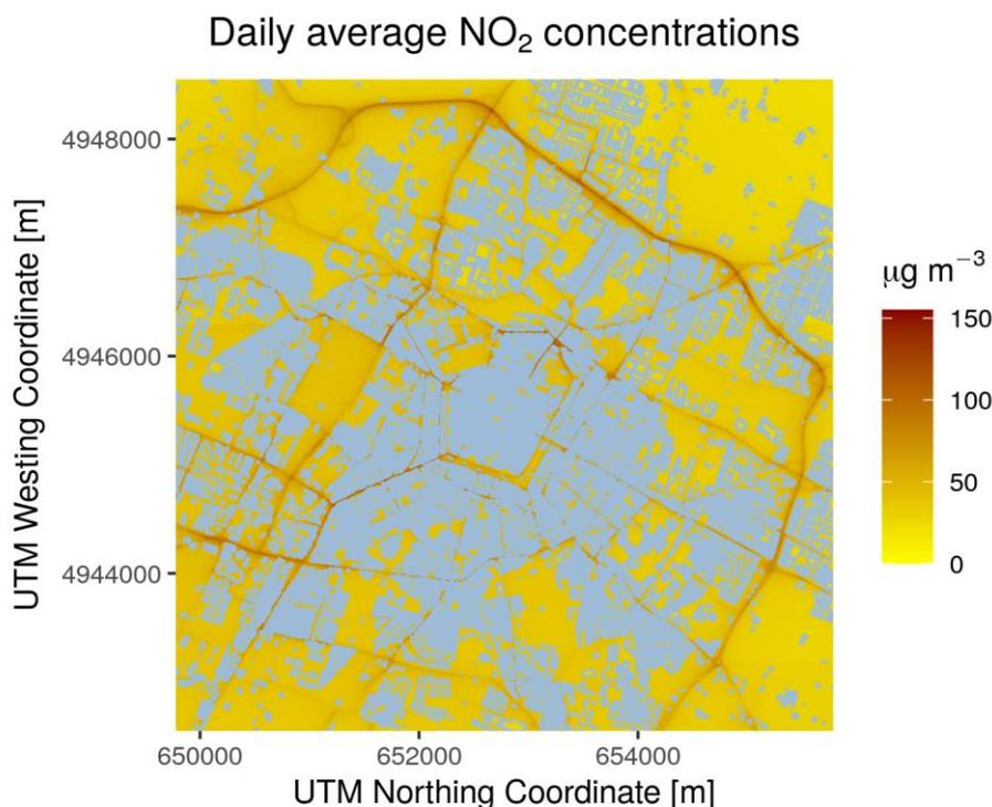
**Figure 1.** Daily average NO<sub>2</sub> concentrations simulated by the hybrid tool composed by the WRF-Chem and the Parallel Micro SWIFT SPRAY modelling suite, for February 18, 2019.
