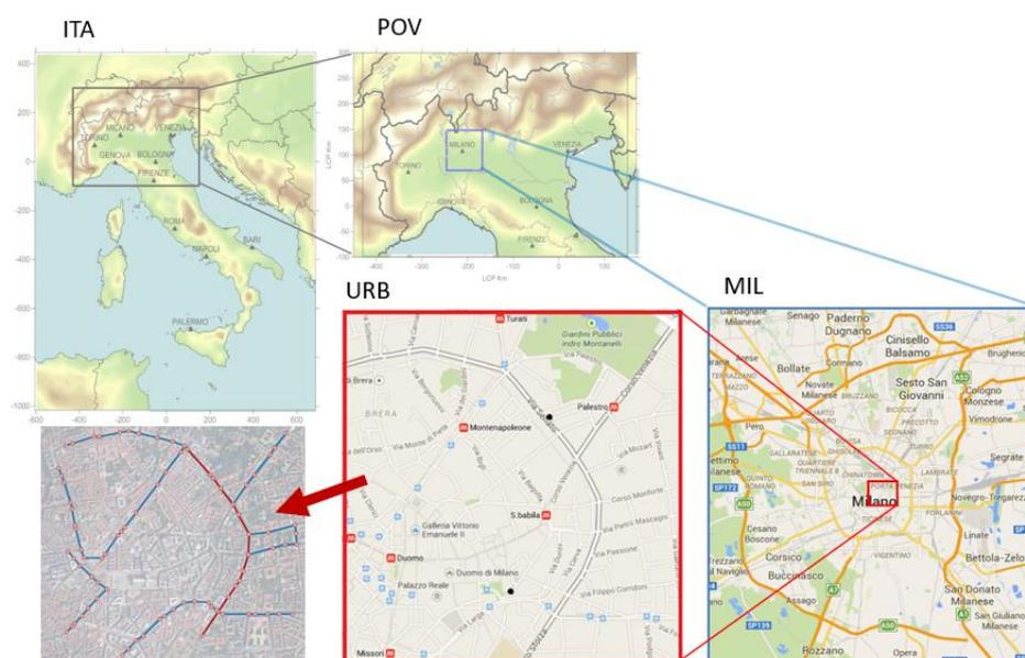
**Figure 1.** CAMx model system of nested domains: ITA, POV, MIL, URB. CAMx-LPiG scheme is implemented in URB domain in a 50 m of resolution sample grid, for the road network shown in the lower left box.
