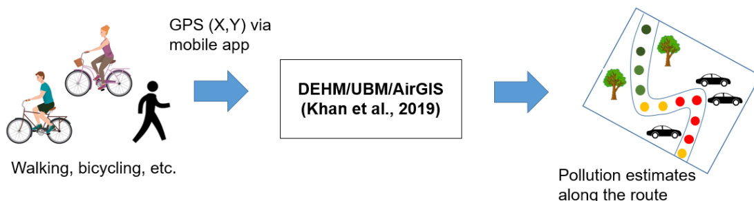
Figure 2: The block diagram of dynamic air pollution exposure modelling framework being implemented in the AirGIS system.
