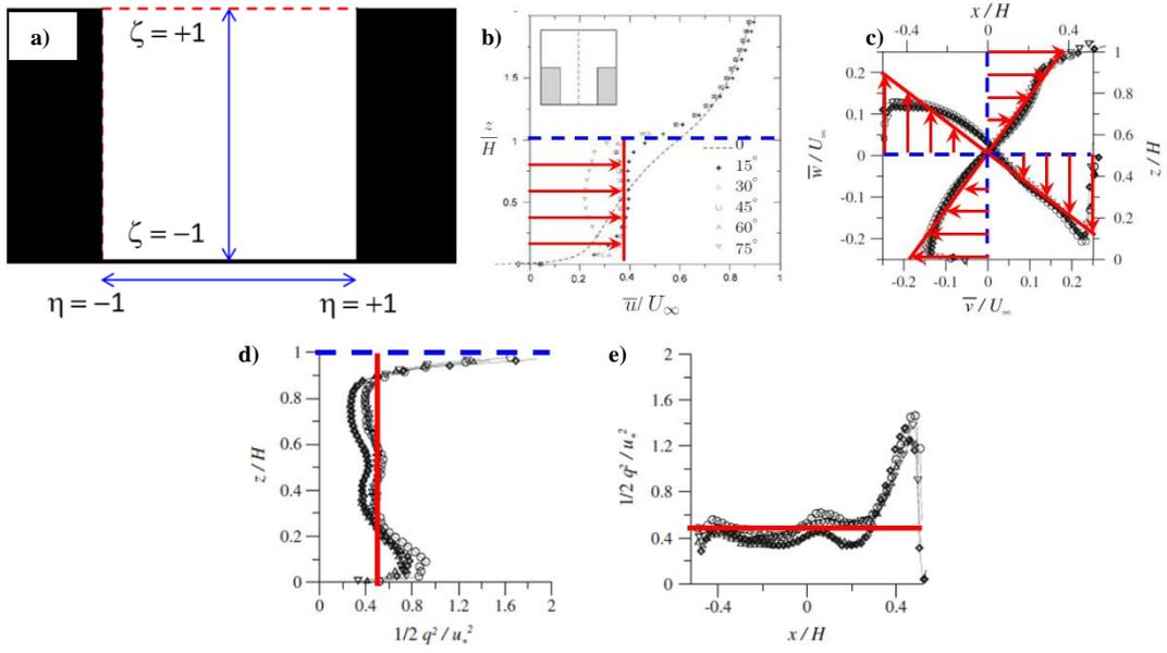
**Figure 2.** Parameterization of the flow in each street: a) local coordinate system, b) longitudinal mean velocity with numerical profiles of Soulhac et al. (2008), c) transverse mean velocity field, d) and e) turbulent kinetic energy, with experimental profiles from Salizzoni et al. (2011).
