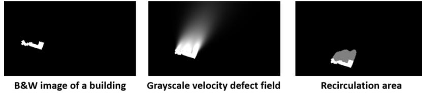
**Figure 3.** Steps of determination of the building recirculation area.
