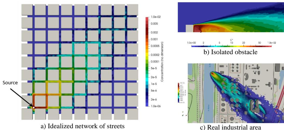
**Figure 5.** Application of the BUILD model on various build-up area types.
