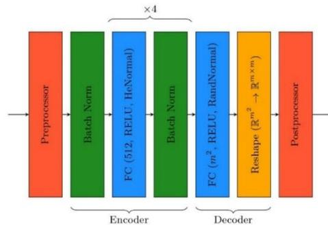
**Figure 2.** Deep Neural Network Architecture for learning atmospheric transport and dispersion from synthetic data.
