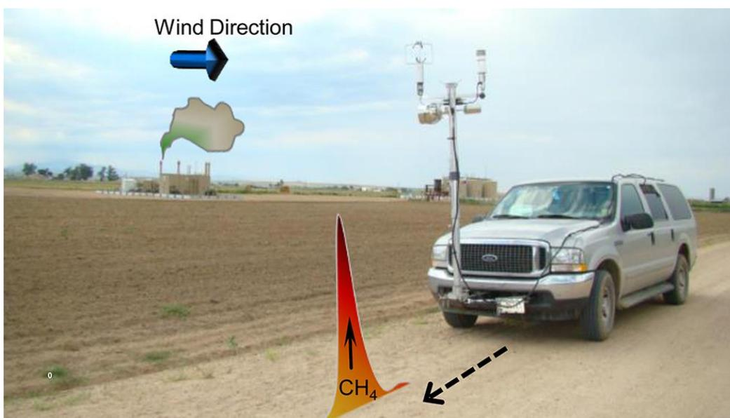
**Figure 1.** Photo from Brantley et al. (2015), showing van and instruments used in their OTM33A source term estimation methodology.
