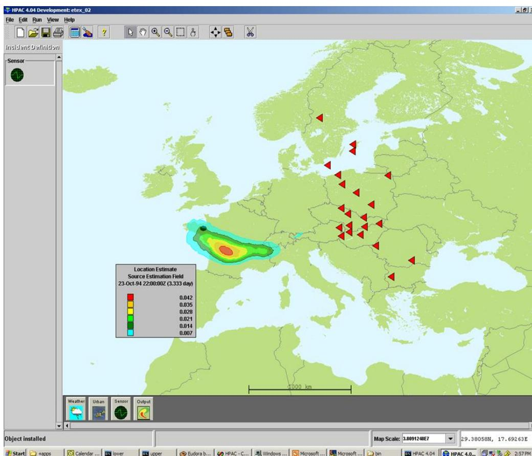
**Figure 3.** SCIPUFF adjoint model predictions of probabilities (color contours) of source location using observations from sensors (triangles) during an ETEX field experiment (from Sykes, 2007). Actual source was at black dot near the NW corner of France.
