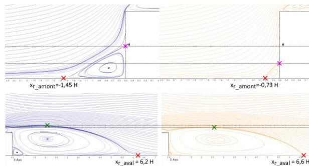
**Figure 4.** Streamlines of the RANS simulation (orange) and the LES simulation (blue), upstream (left) and downstream (right) of the obstacle
