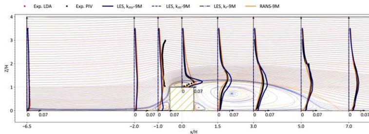
**Figure 6.** Evolution of dimensionless turbulent kinetic energy ( $k/U_\infty^2$ ) along the domain from the experiment (dot red and black), the RANS simulation (orange line) and the LES simulation (blue line). In the background, streamlines from Figure 3 with the RANS simulation (orange) and the LES simulation (blue)
