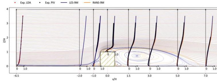
**Figure 5.** Evolution of  $U/U_\infty$  along the domain from the experiment (dot red and black), the RANS simulation (orange line) and the LES simulation (blue line). In the background, streamlines from Figure 3 with the RANS simulation (orange) and the LES simulation (blue)
