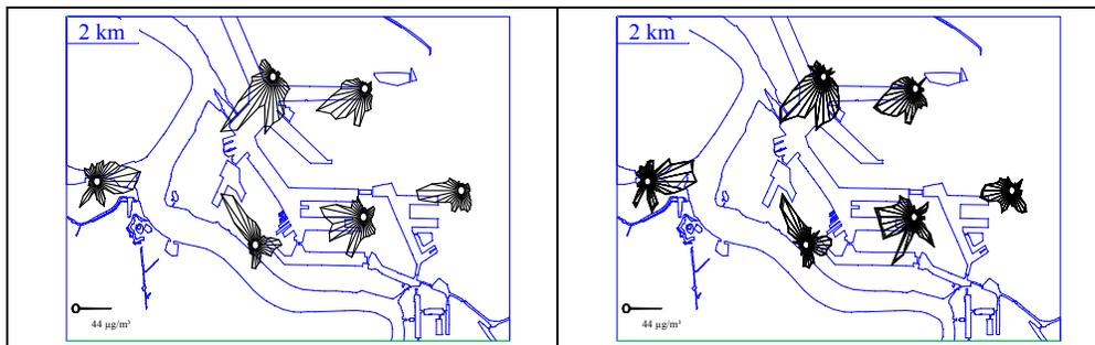
Figure 1. Pollution roses for the Antwerp harbour, 1997. Left: calculated from half hourly SO<sub>2</sub>-concentrations. Right: Calculated from 24-hour averaged SO<sub>2</sub>-concentrations.
