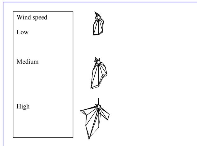
Figure 3. Pollution roses for three wind speed classes. Pollutant Pb, measured near a lead smelter, years 1996-1997.
