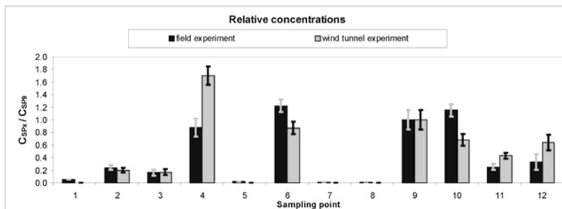
Figure 4. Relative concentrations (referred to SP9), comparison of field and wind tunnel experiment. The error bars are derived from 30 minutes averages (full scale).
