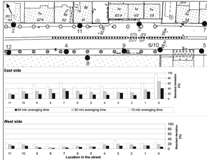
Figure 3. Distribution of concentration standard deviations in the street canyon for different averaging times. Measurement points east side: light grey dots, west side: dark grey dots. The numbered black dots represent the sampling points in the field experiment.
