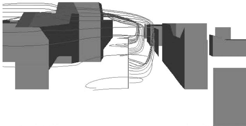
*Figure 3. Simulation of a tracer experiment in an urban street canyon with MITRAS. Buildings are indicated as shaded blocks. The tracer is released at a line source in the centre of the street. Advection of the tracer is visualised by streamlines. Above the urban canopy, the wind is blowing from right to left (Schluenzen, 2002).*
