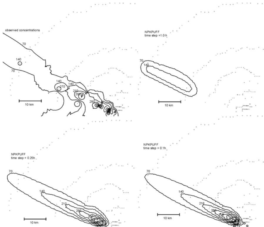
**Figure 1. Day sums (ppt.h) for observed concentration and modelled concentration in air by NPK-PUFF using time steps of 1h, 0.25h and 0.1h for Kincaid day 16-05-1981.**
