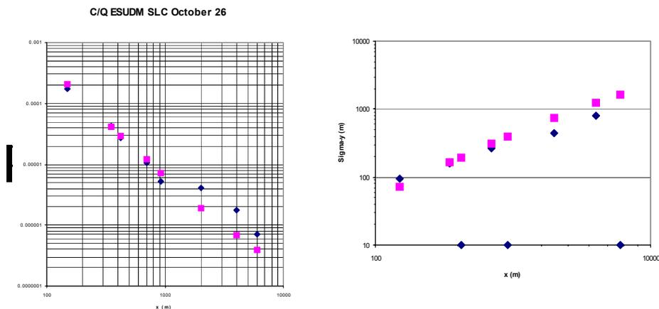
Figure 3. ESUDM predictions (squares) and observations (diamonds) of (left panel) maximum 30-minute average  $SF_6$  C/Q and (right panel)  $\sigma_y$  during a two-hour experiment duration as a function of distance averaged over the three 26 October 2000 nighttime SLC tests.
