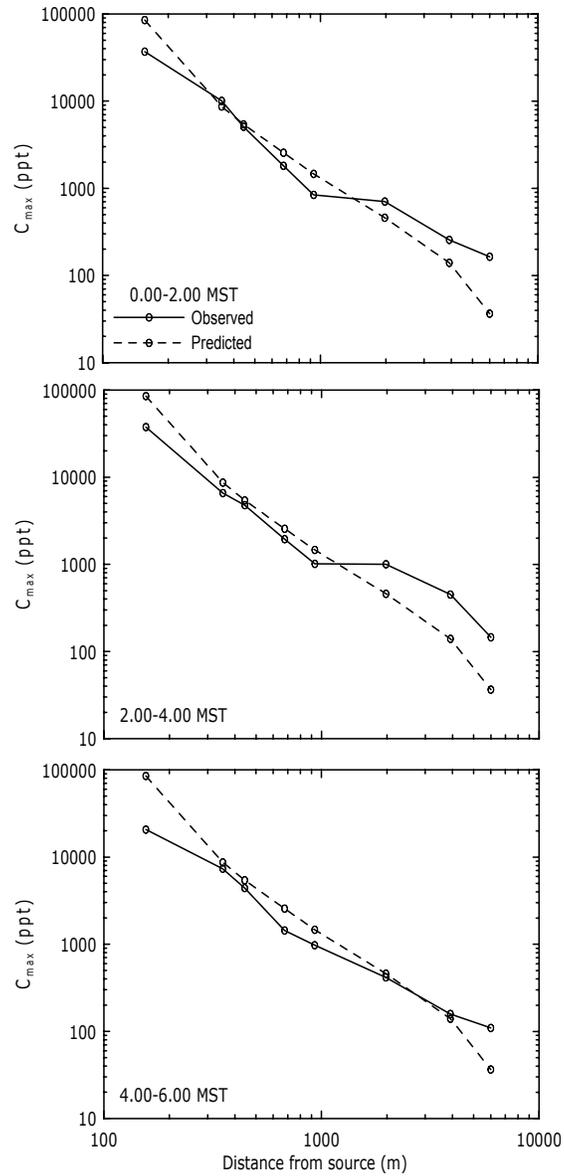
Figure 2. ASUDM predictions (dashed lines) and observations (solid lines) of maximum 30-minute average  $SF_6$  concentration (ppt) during a two-hour experiment duration as a function of distance for three 26 October 2000 nighttime tests in SLC.
