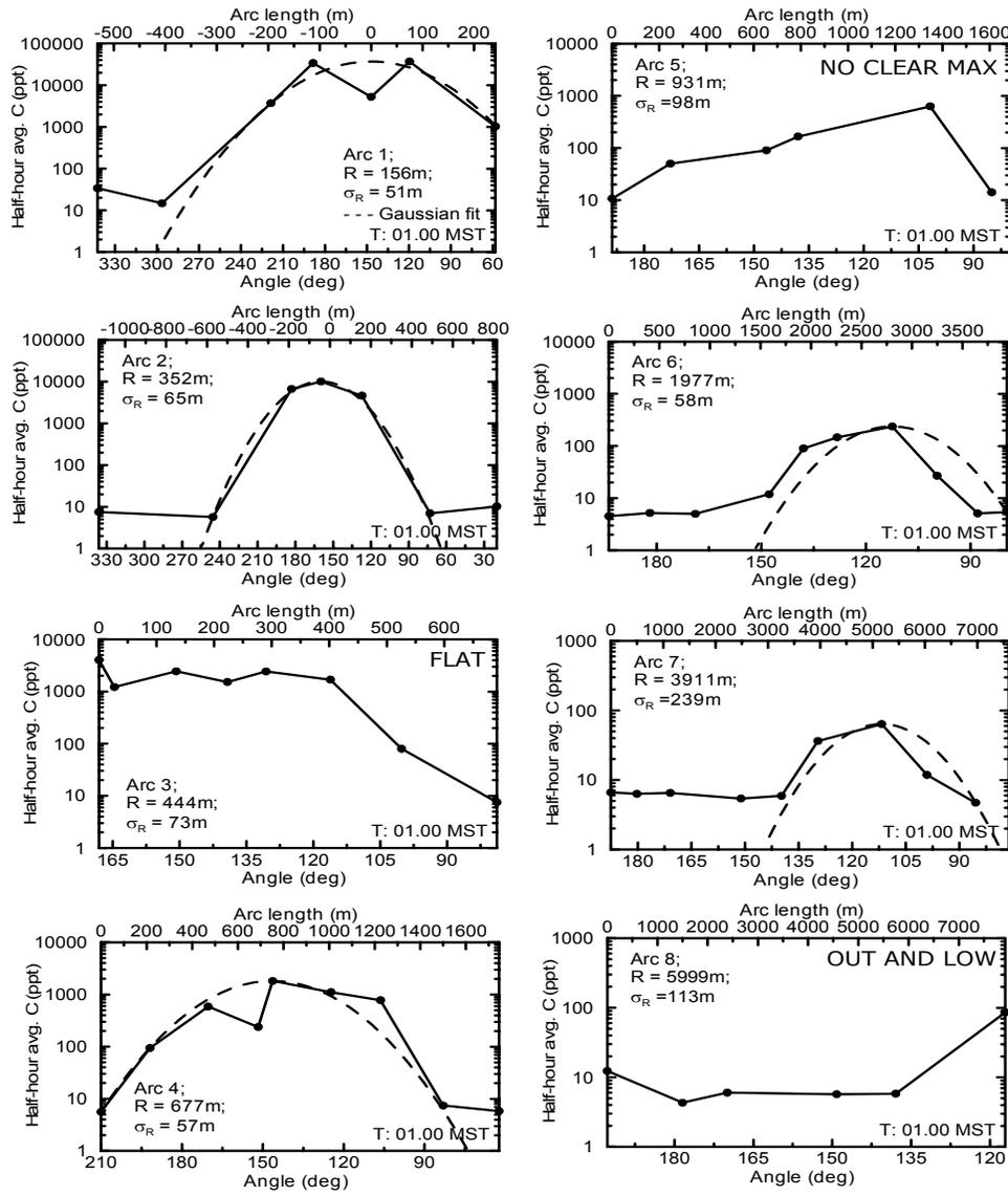
Figure 1. Observed concentrations (in ppt for 30 minute averages) on eight sampling arcs for the 26 October 00 MST SF<sub>6</sub> release during the Salt Lake City Urban 2000 experiment. The arc number and its distance, R, from the source are given, as well as the  $\sigma_R = \sigma_y$  value best fit using the dashed Gaussian curve.
