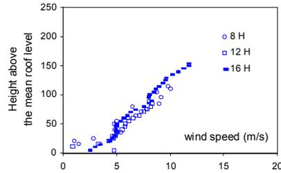
Figure 6. Vertical profiles of the horizontal wind speed observed at the urban station during one day with stable direction.
