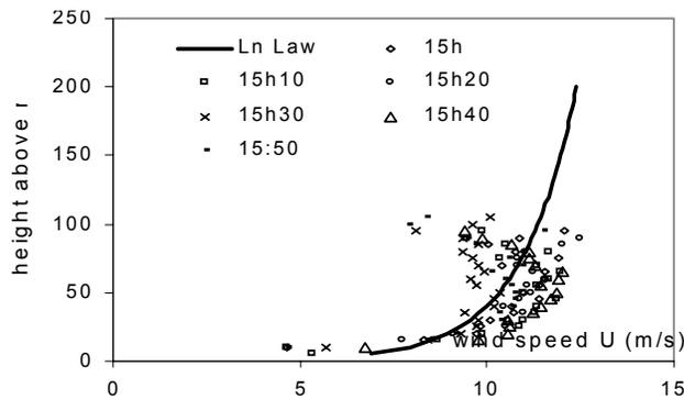
Figure 8. rural site: Ln law profiles obtained using the optimised parameters  $u^*=0.6$  m/s and  $z_0=0.05$  m, compared to observed values. The displacement height  $d=0$  m
