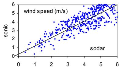
Figure 2. Mean wind speed, comparison sodar /sonic at the rural station.
