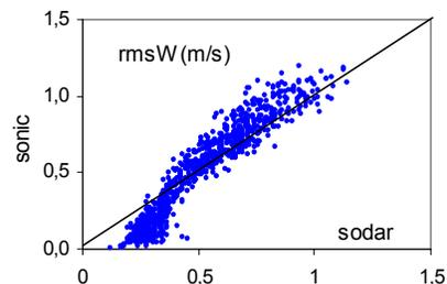
Figure 4. rms value of the vertical wind speed W, comparison sodar /sonic at the rural station.
