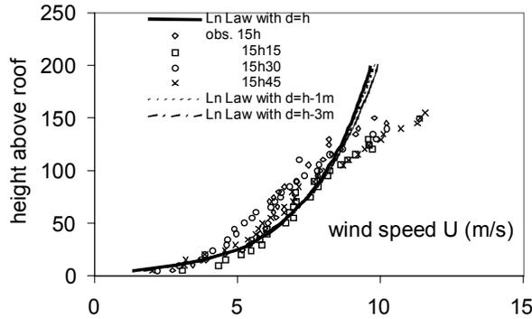
Figure 7. urban site: Ln law profiles obtained using the optimised parameters  $u^*=0.91$  m/s and  $z_0=2.8$  m, compared to observed values. Three displacement heights have been used  $d=h$ ,  $h-1m$  and  $h-3m$ ,  $h$  being the building height.
