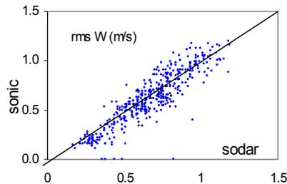
Figure 3. rms value of the vertical wind speed W, comparison sodar (fifth level)/sonic at the urban station.
