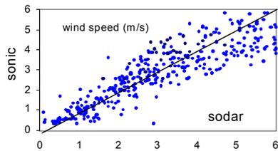
Figure 1. Mean wind speed, comparison sodar (fifth level)/sonic at the urban station.
