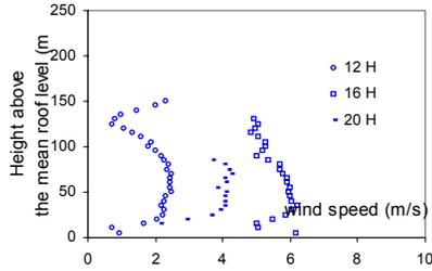
Figure 5. Vertical profiles of the horizontal wind speed observed at the urban station during one day with large wind direction variations.
