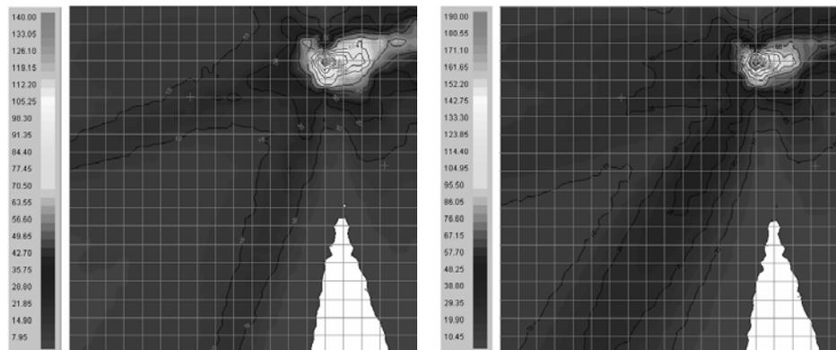
*Fig. 3a, 3b. AERMOD and RAMS-AERMOD maximum predicted 1-hr concentrations*
