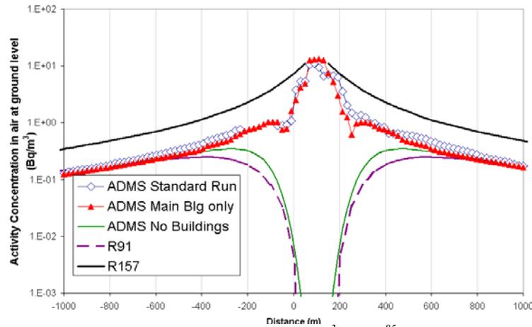
Figure 2. Predicted activity concentrations in air ( $Bq\ m^{-3}$ ) of  $Kr^{85}$  along a line through the 50m stack at Dungeness (see Figure 1b-line is along the edge of buildings B4 and B2 and through building B9)
