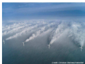
Wake effects on an offshore wind farm (WRAPP)
