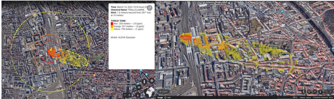
Figure 3: Threat zone, based on the thresholdvalues, calculated with ALOHA (left) with LASAT (1st run - flat, without buildings, right) for the accident release scenario at Graz train station. (Map data ©2022 Google)
