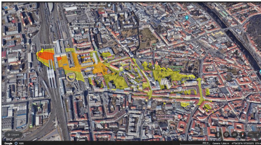
Figure 4. Threat zone, based on the thresholdvalues, calculated with LASAT (2.nd run – with terrain) for the accident release scenario at Graz train station (Map data ©2022 Google)
