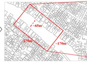
Sketch of the Canal Grande portion geometry considered in CFD simulations
