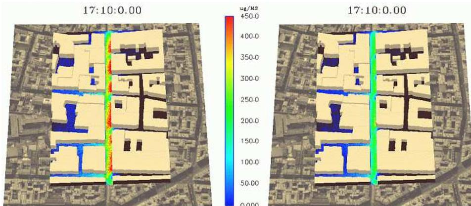
Figure 2: Illustration of the "Street Canyon" geometry (without TiO<sub>2</sub> on the left, with TiO<sub>2</sub> on the right).
