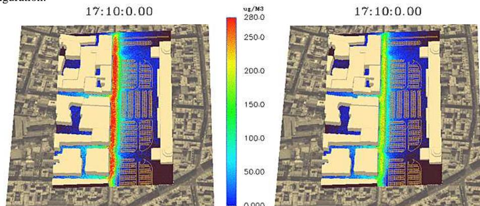
Figure 3: Illustration of the "Street without vis-a-vis" geometry (without TiO<sub>2</sub> on the left, with TiO<sub>2</sub> on the right).
