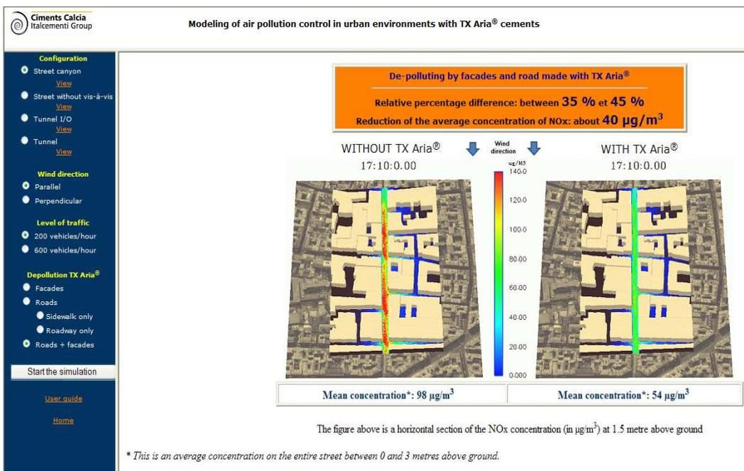
Figure 7: Snapshot of the working Web page of EXP' AIR. Selection of cases and controls are grouped on the left side of the page.
