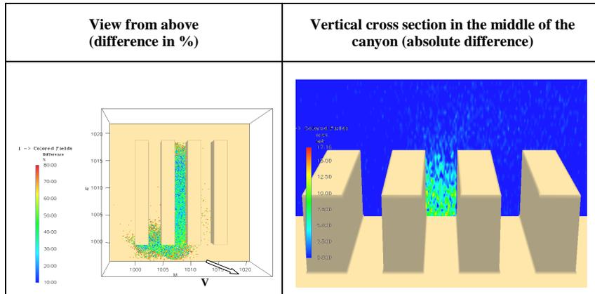
with the same order of magnitude as found in the measurements. In the scenarios that best demonstrate the pollution abatement effect of the photo-catalytic coating, the efficiency of the TiO<sub>2</sub> coating varies in the range 15% to 50% in the measurements and in the range 35% to 50% in the modelling simulations.
