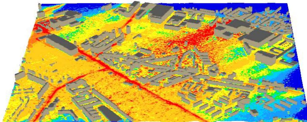
Figure 6: Snapshot of a realistic district simulation with MSS included into EXP’AIR (digital data for Berlin provided by WEST Sustainability and Virtual City Systems)
