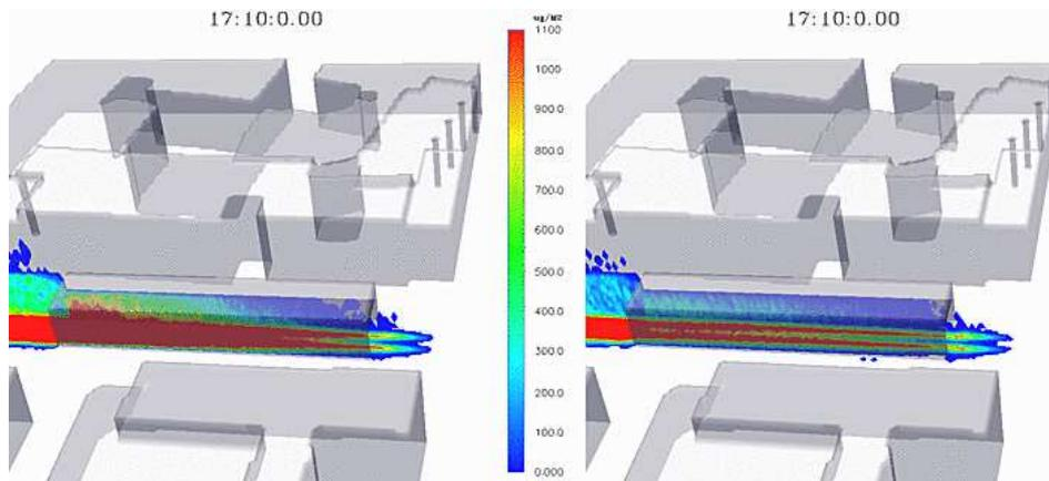
Figure 5: Illustration of the “Tunnel” geometry (without TiO2 on the left, with TiO2 on the right).
