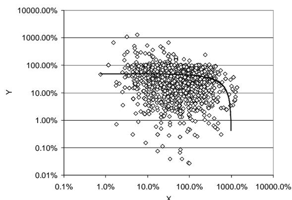
Figure 2. Diagram of modules of relative errors (Y) vs. relative flows (X). Relative flows are expressed with respect to the network average value; the black line shows the linear fitting.
