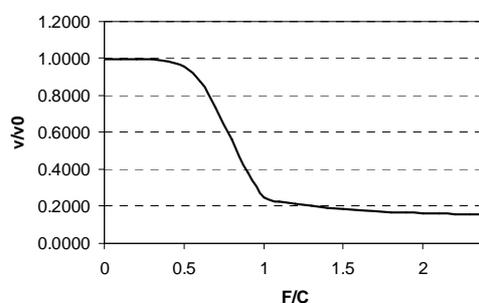
Figure 1. Speed function –  $v/v_0$  : real versus free-flow speed ratio; F/C : traffic flow versus road capacity.
