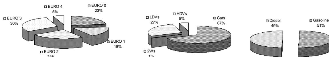
Figure 5. Tunisia 2006 vehicle fleet distribution per emission standards (left), categories (centre) and fuel (right).
