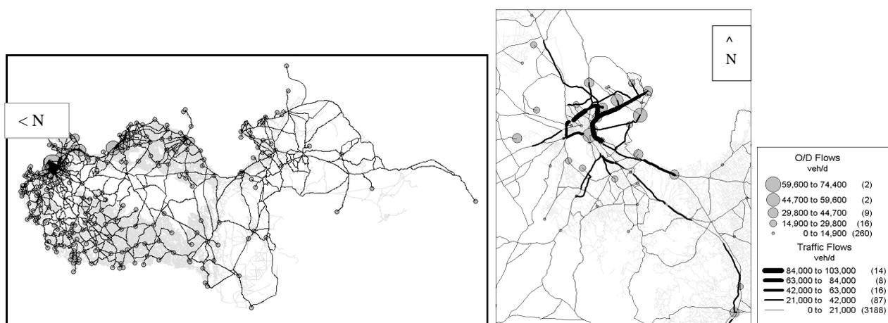
Figure 3. Traffic simulation results at national scale (left) and city scale (Tunis, right).
