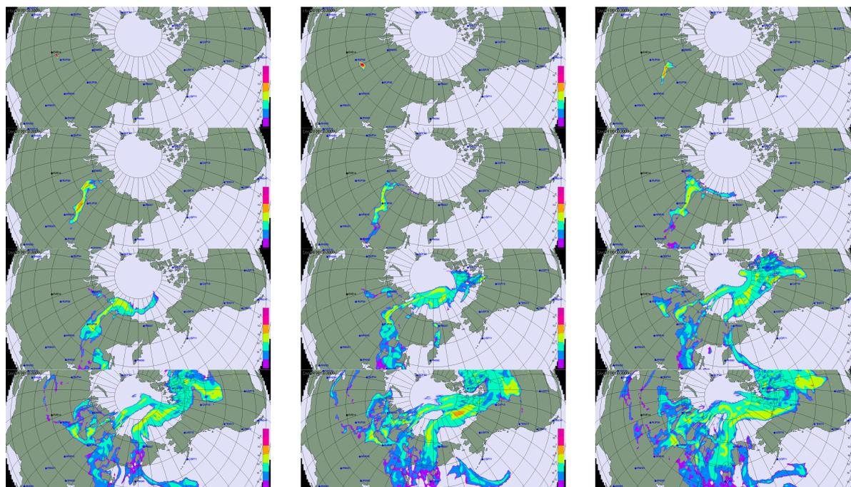
Figure 1. Snapshots of the results of a forward atmospheric transport model (courtesy of ZAMG) giving rise to the fictitious scenario of radionuclide detections presented in Table 1. The snapshots are organised row-wise and the time interval separating two successive plots is 24 hours. The first snapshot (top left-hand corner) illustrates the shape of the plume at 00 UTC on 29 November, the last one at 00 UTC on 10 December 2009 (bottom tight-hand corner).
