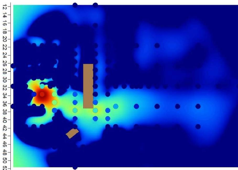
Figure 1. Experimental values of deposited activity (qualitatively, in log scale) and the layout of obstacles.
