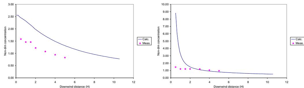
Figure 8. Comparison of calculated and measured non-dimensionalized concentration in the along-wind direction, downwind of the obstacle, at ground level, for source located at the downwind side: Cube, (left), cylinder, (right)
