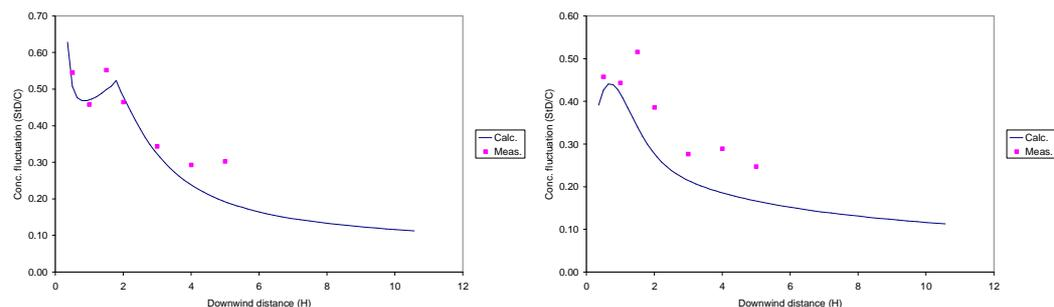
Figure 9. Comparison of calculated and measured concentration fluctuation intensity in the along-wind direction, downwind of the obstacle, at ground level, for source located at the downwind side: Cube, (left), cylinder, (right)
