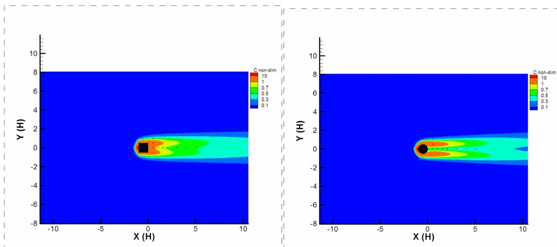
Figure 3. Contour plots of calculated non-dimensionalised concentration on the horizontal plane at the height of the gas source, located at the upwind face of the obstacle: cube (left), cylinder (right)
