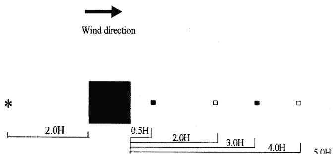
Figure 1. Plan view of the basic experimental configuration involving a single cube, with the source located  $2.0H$  upwind (\*: source, ■: detectors).
