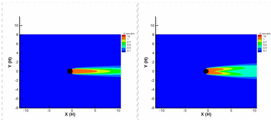
Figure 4. Contour plots of calculated non-dimensionalised concentration on the horizontal plane at the height of the gas source, located at the downwind face of the obstacle: cube (left), cylinder (right)
