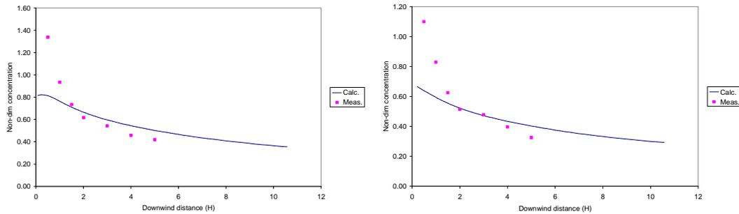
Figure 6. Comparison of calculated and measured non-dimensionalized concentration in the along-wind direction, downwind of the obstacle, at height H/2, for source located 2H upwind: Cube, (left), cylinder, (right)
