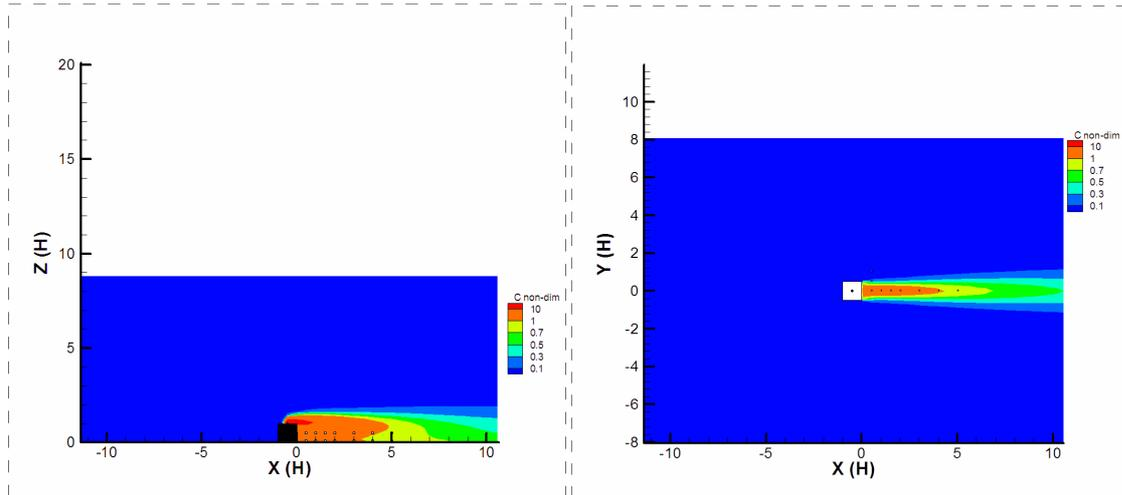
Figure 5. Contour plots of calculated non-dimensionalised concentration for the gas source located on top of the cubical obstacle: vertical plane (left), horizontal plane at the height of H/2 (right)
