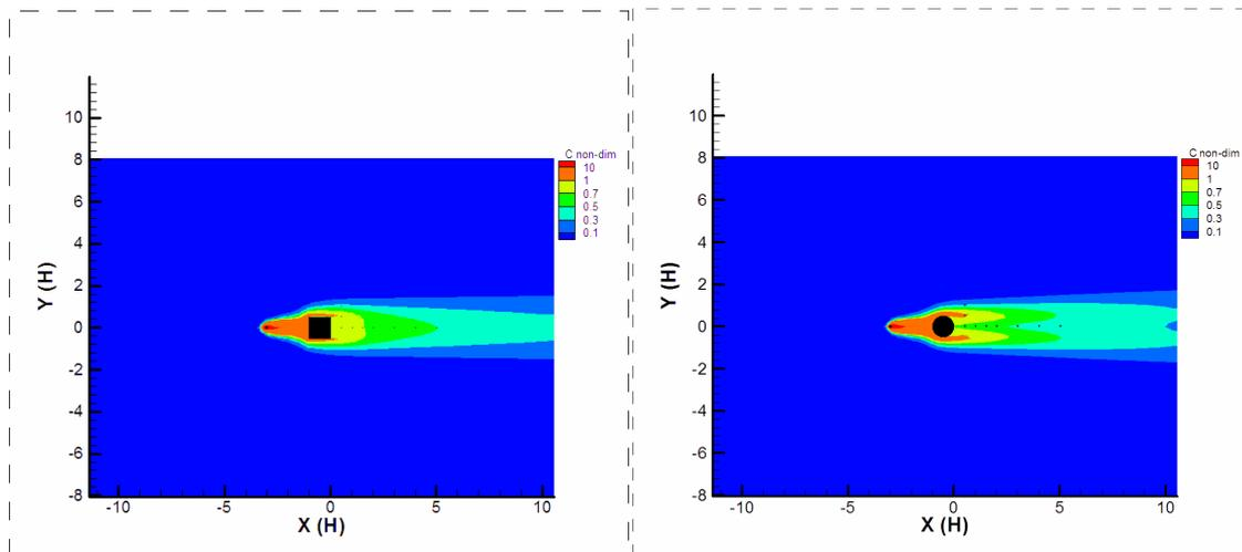
Figure 2. Contour plots of calculated non-dimensionalised concentration on the horizontal plane at the height of the gas source, located at a distance of  $2H$  upwind of the obstacle: cube (left), cylinder (right)
