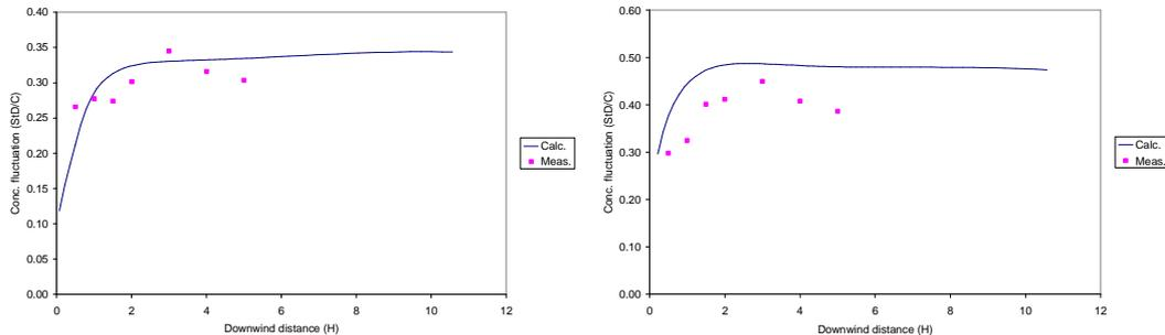
Figure 7. Comparison of calculated and measured concentration fluctuation intensity in the along-wind direction, downwind of the obstacle, at height H/2, for source located 2H upwind: Cube, (left), cylinder, (right)
