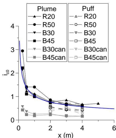
Figure 5. Evolution of  $i_{c0}$  in the wind direction for every experimental configuration. The blue curve was obtained thanks to Equations (5).
