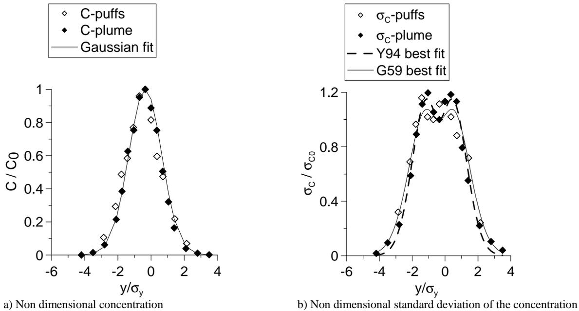
Figure 4. Typical results for plume and puffs in the R20 configuration: a) Non dimensional concentration distribution, b) Non dimensional standard deviation of the concentration. Y94 and G59 denote respectively the fit laws derived from analytical relations given in Yee *et al.* (1994) and Gifford (1959).
