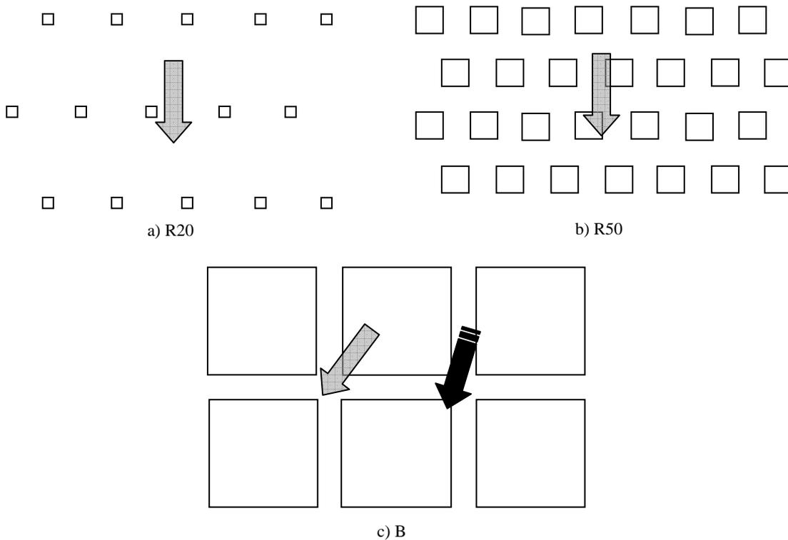
Figure 3. The different configurations tested during the wind tunnel experiments: a) rough surface with 20 mm cubic roughness elements (R20), b) rough surface with 50-mm cubic roughness elements (R50) and c) idealized urban area (UA). The grey arrows indicate the wind direction in each experiment. Note that two wind directions were tested for the B configuration: 30° (configuration B30, black discontinued arrow) and 45° (B45 grey arrow)
