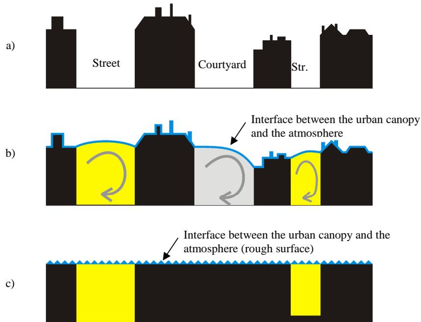
Figure 1. Description and simplified representation of an urban district in SIRANERISK: a) cross section of the real topography, b) visualisation of the interface between the atmosphere and the urban canopy and c) representation of the district in SIRANERISK
