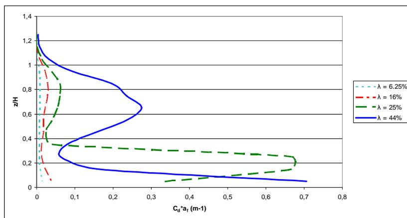
Figure 1: Product of sectional drag coefficient and frontal density per volume as function of the altitude for various packing densities.
