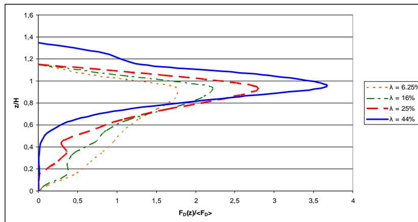
Figure 3: Vertical profile of drag force per volume normalized by the mean drag force, comparison of the 4 densities.
