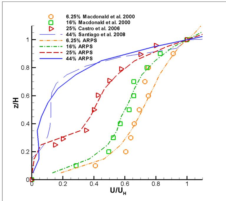
Figure 2: Normalized vertical velocity profiles for the 4 densities
