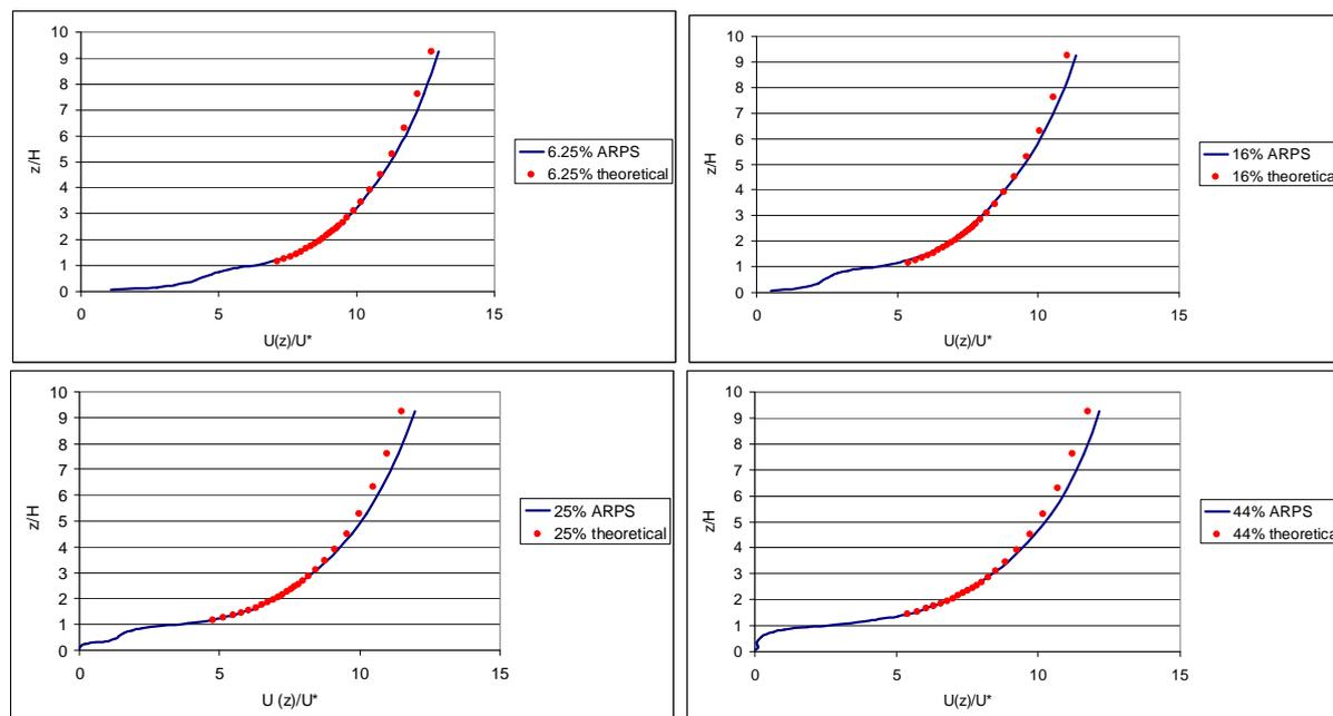
Figure 4 : Comparison of the longitudinal velocity profile computed by ARPS and a theoretical logarithmic profile with same roughness parameters: a)  $\lambda = 0.625\%$ , b)  $\lambda = 16\%$ , c)  $\lambda = 25\%$ , d)  $\lambda = 44\%$ .
